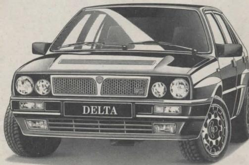
Delta HF integrale 8V, Turbolader, 177 PS (130 kW).
