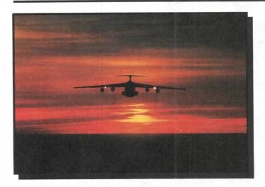
Length: 247 feet 10 in Wing Span: 222 feet 8 1/2 in Height: 65 feet 1 1/2 in Weight: Gross: 837,000 lbs Speed: Max 571 mph
